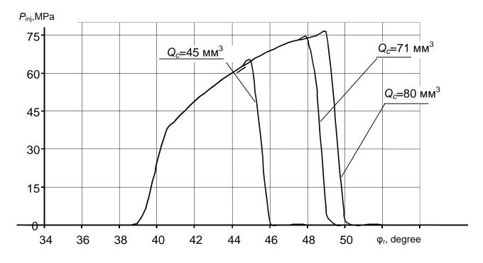
Fig. 4. The Dependence of injection pressure  $P_{inj}$  on the angle of the pump shaft rotation ( $n_r=2000 \text{ min}^{-1}$ ,  $\varphi_{op}=37^{\circ}$ )
