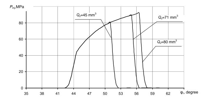
Fig. 5. The Dependence of injection pressure  $P_{inj}$  on the angle of the pump shaft rotation ( $n_r=3000 \text{ min}^{-1}$ ,  $\varphi_{op}=40^{\circ}$ )
