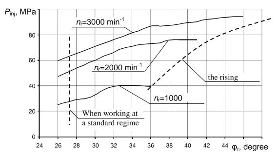
Fig. 2. The Dependence of the maximum pressure of the injection fuel  $P_{inj}$  on the angle of valve opening  $\varphi_{open}$
