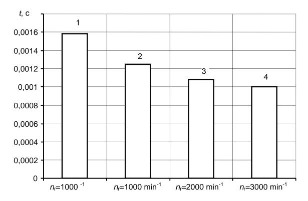
Fig. 8. Injection Duration of Fuel feeding depending on the shaft rotation frequency of the pump for the systems: 1 - standard (traditional), 2,3,4 - experimental
