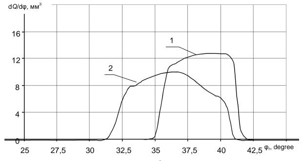
Fig. 7. Differential characteristics of fuel feed  $n_r=1000 \text{ min}^{-1}$ : 1 – the experimental system, 2 – the standard system
