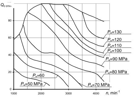
Fig. 1. The dependence of optimal pressure  $P_H$  in the accumulation system "Common Rail" on the engine shaft rotation frequency and the relative cycle feed Q concerning the Diesel Mercedes OM611 [1]
