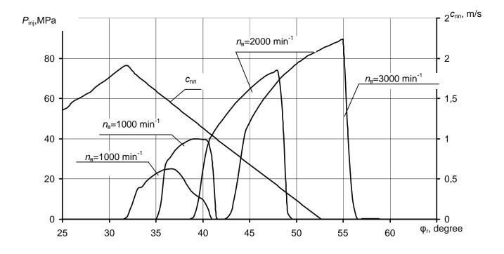
Fig. 6. The Dependence of injection pressure  $P_{inj}$  and the plunger speed on the angle of the pump shaft rotation  $\varphi_{shaft}$  at  $Q_c=71 \text{ mm}^3$
