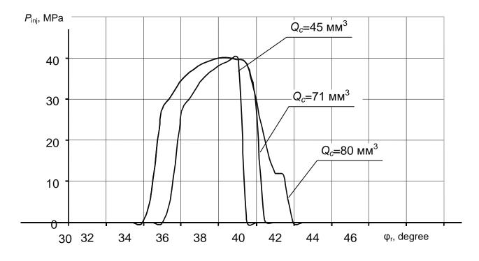
Fig. 3. The Dependence of injection pressure  $P_{inj}$  on the angle of the pump shaft rotation  $(n_{shaft}=1000 \text{ min}^{-1}, \varphi_{op}=34^{\circ})$
